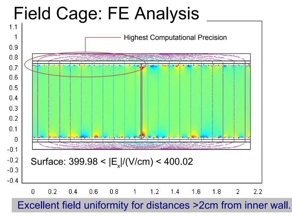
Finite element analysis done using FEMLAB (comsol.com)
