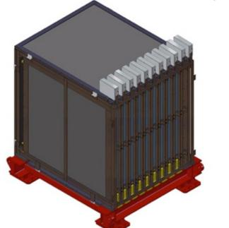
scintillator bars/WLS fiber /iron layers/ Hamamatsu MPPC readout
