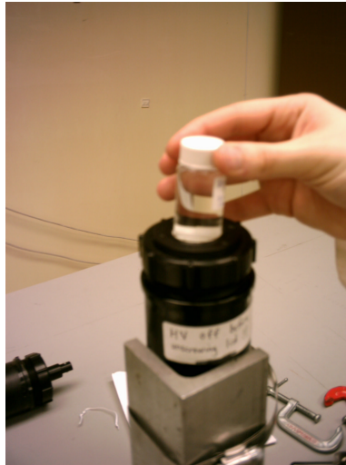
Figure 5: Loading Scintillation Counting Vial into Apparatus
