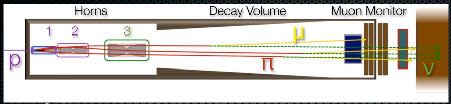
30 GeV protons hit graphite target
