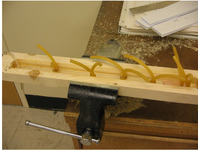
Figure 3.7: Mould used to seal the bottom end of prototype B. It is made of wood, a material that turned out to be quite terrible for this purpose. Plastic tubes are configured in such a way that they will interconnect all the panel pieces together once the sealing procedure is completed.
