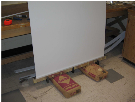
Figure A.3: 1-cm thick aluminum mould used to seal both ends of prototype C. This prototype consisted of a single complete Matraplast panel.
