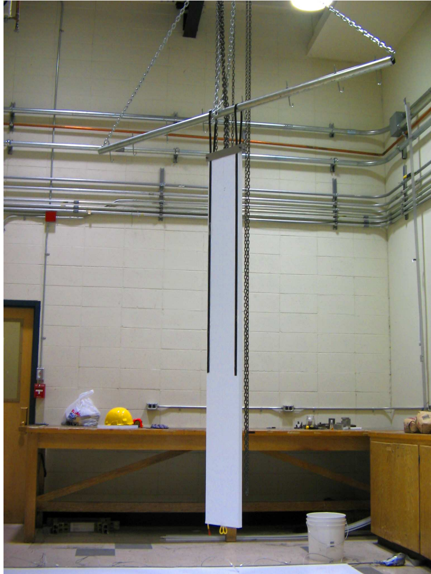
Figure 3.6: Prototype A hanging off the crane and supported by long metal straps epoxied onto the surface. The panel has been completely filled with water and remained in this position over a period of two months without showing any sign of leakage.
