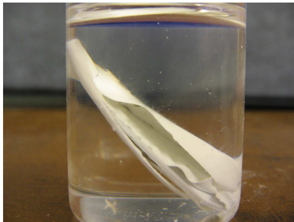
Figure A.4: Three coats of paint peeling off the plastic surface at a temperature of 35°C. The primer used in this case was Krylon.
