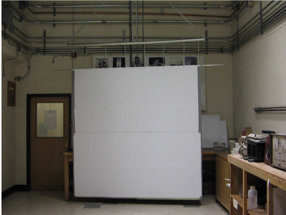
Figure 2.9: Full-sized detector filled with sand. The various panels have been glued to one another using contact cement as well as double sided tape. The whole structure has been hanging in the lab over a total period of 6 months.
