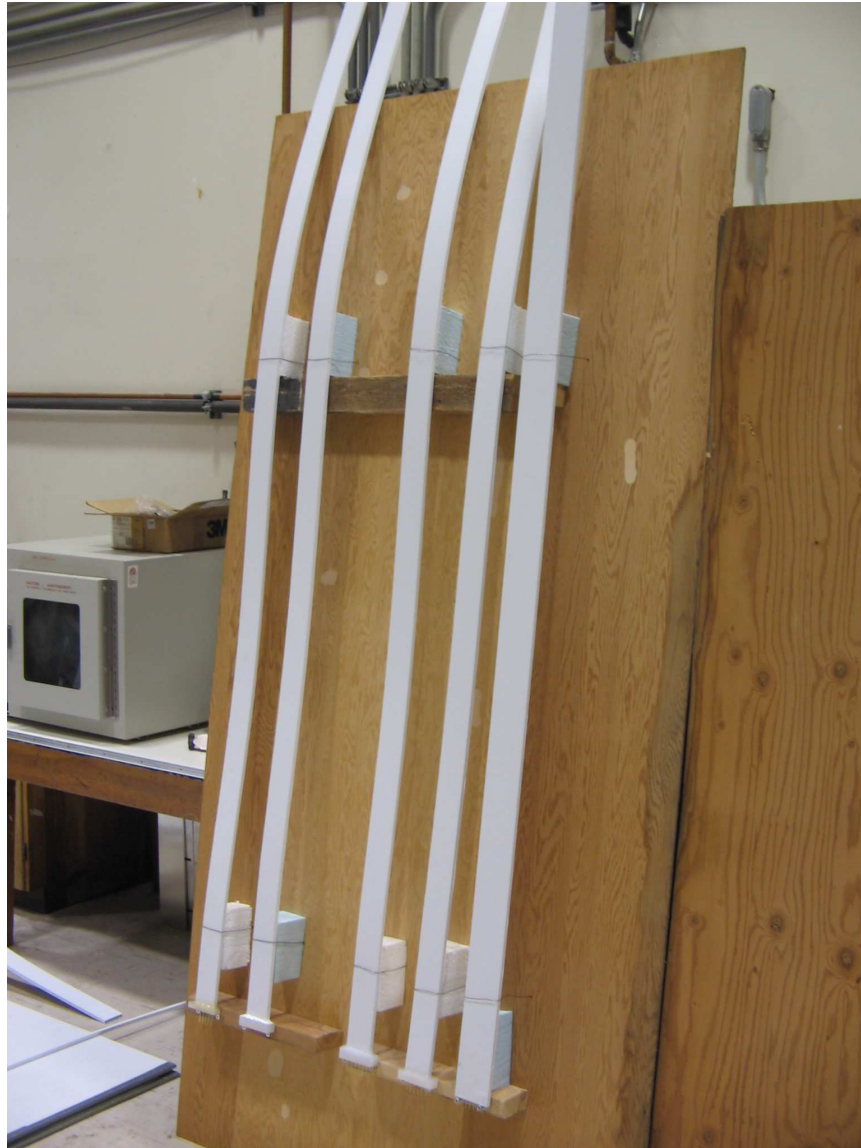
Figure A.1: First series of passive sealing tests using endcaps glued to Matraplast panels by mean of RTVs and epoxies.
