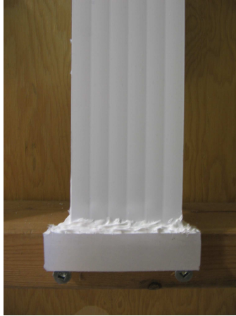
Figure 3.1: Passive water endcap sealed with white RTV
