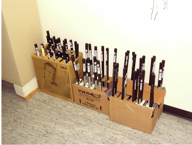
Figure 4.8: A total of 32 samples have been built for long term tests with liquid scintillator
