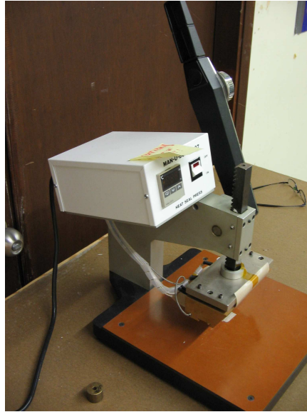
Figure 3.2: Small press used to thermally weld endcaps to the Matraplast panels. The press allows one to apply a constant pressure with a pointed metal piece heated up to the polypropylene melting point.
