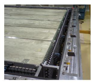
Figure 1.4: The uncovered FGD in a horizontal position. The scintillator panels can be see in the center of the image, and the MPPCs attached to the black daughter card and bus-boards seen in black surrounding the scintillator layers.(Permission pending)
