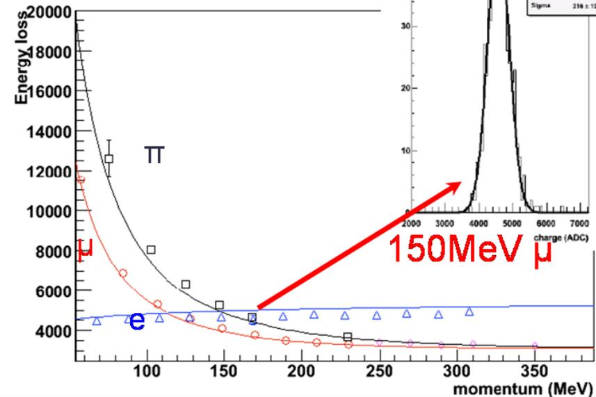
>5 $\sigma$  separation of e/ $\mu$  for p>200MeV
