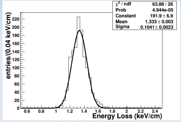
Energy loss distribution for negative particles with 400 < p (MeV/c) < 500
