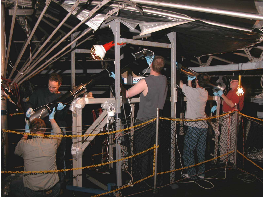
Figure 3.16: Example of the step-by-step insertion procedure used to fit the manipulator into the 1KT. Here the second part of the vertical section is lifted off the makeshift assembly table, before it can be lowered into the detector.
