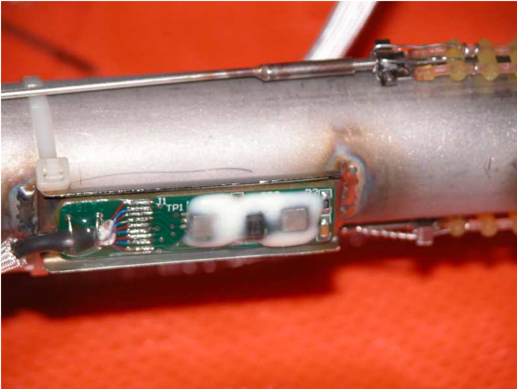
Figure 3.5: The inclinometer board holding the Limit and Safety inclinometers for the B-Arm. The board is mounted on a holder welded to the arm. The board is coated with polyurethane to make it water resistant. Some extra epoxy coating was added for additional safety.
