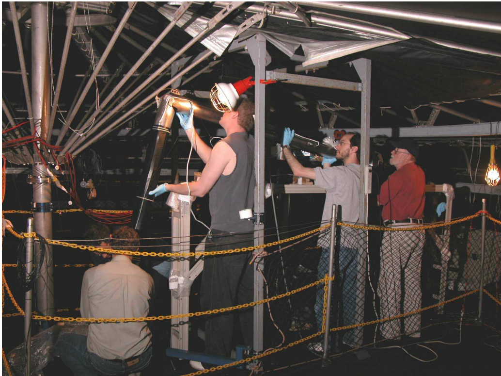
Figure 3.17: The stage of the manipulator insertion that is most critical, fitting the VS pieces into the CRP under the roof support.
