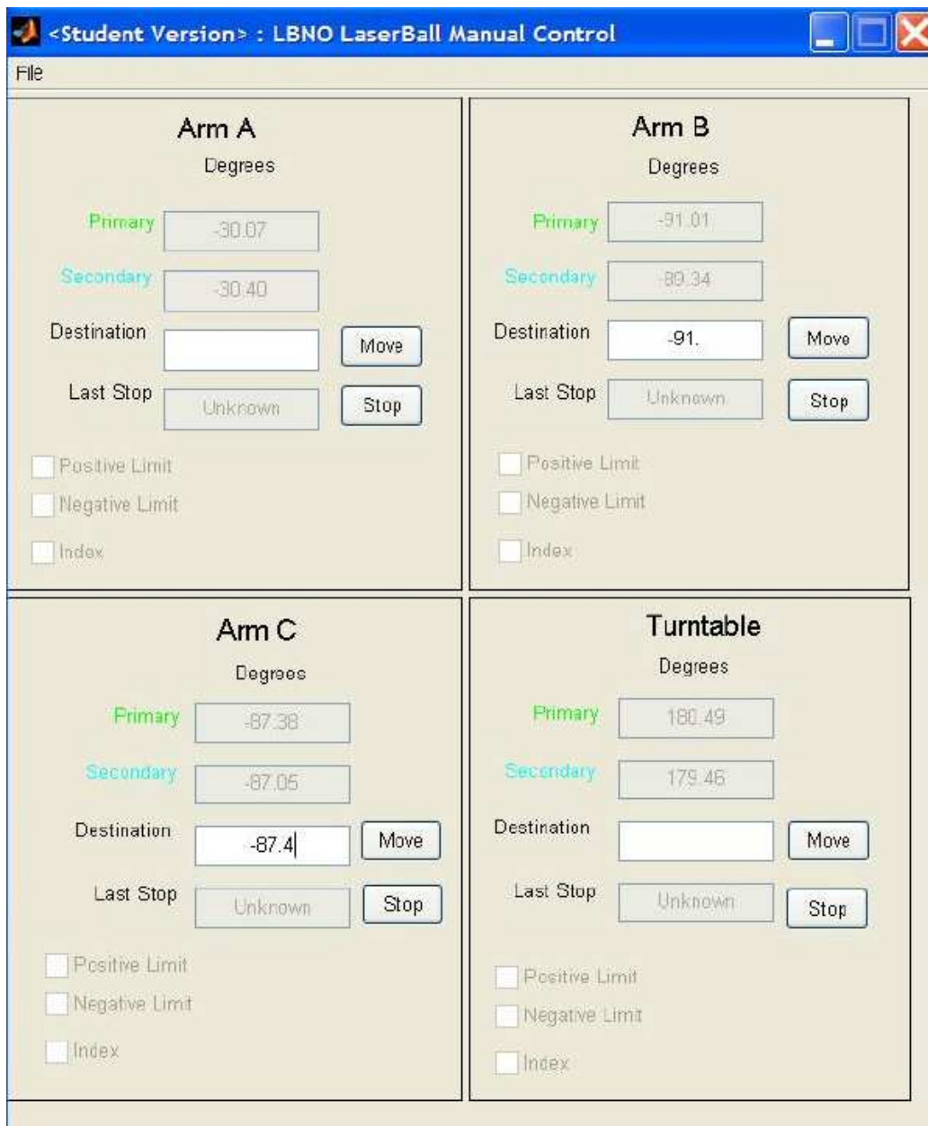
Figure 3.10: The Manual Control GUI for the Manipulator. This GUI allows the user to move one arm to a specific angle.
