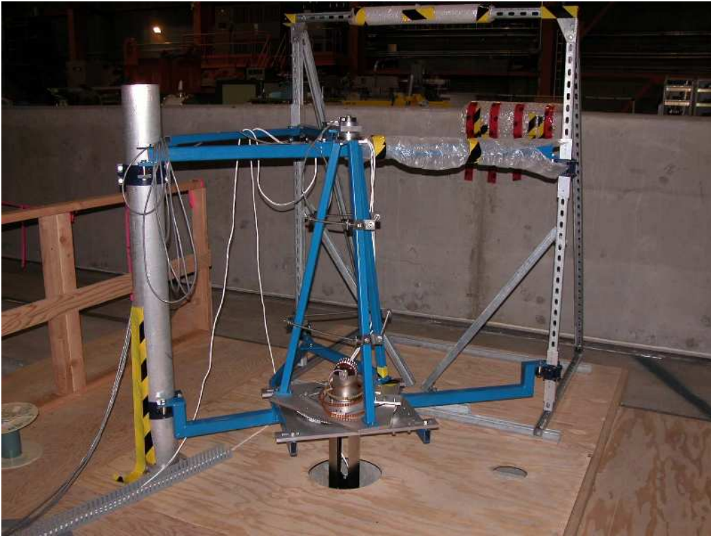
Figure 3.11: Mockup of the 1KT access at TRIUMF. The support structure for the manipulator is set up on imitations of the roof support beam and the CRP cage. The weight of the Manipulator is on the joint at the top of the tripod. The tripod holds the turntable and manipulator in place.
