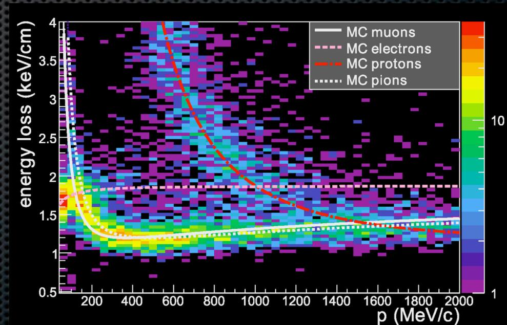
Sample of positively charged particles produced in neutrino interactions.
