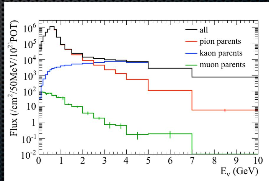
$\nu_\mu$  flux broken down by parent that produces  $\nu$
