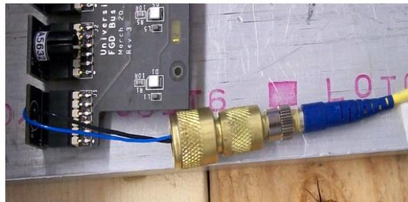
Figure 1.8: A photograph of the MPPC coupler which allows an FC cable to couple directly to an MPPC attached to a daughter board.
