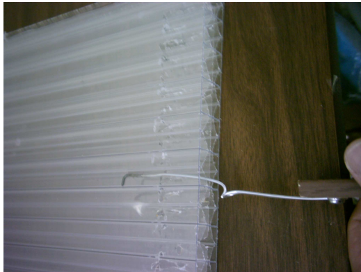
Figure 2: Photo of puncturing holes in polycarbonate partition walls
