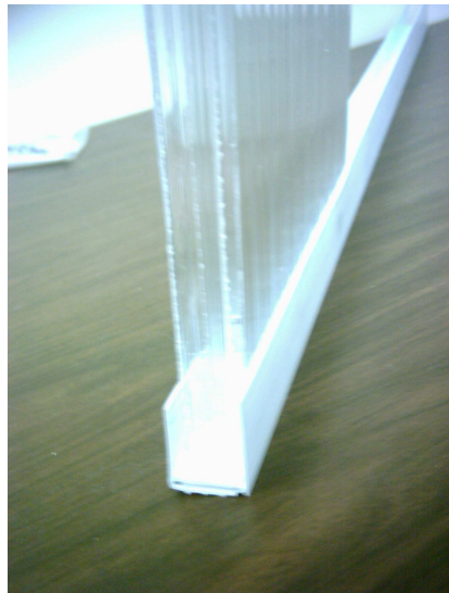
Figure 3: Photo of polycarbonate paneling with the mold on the bottom.
