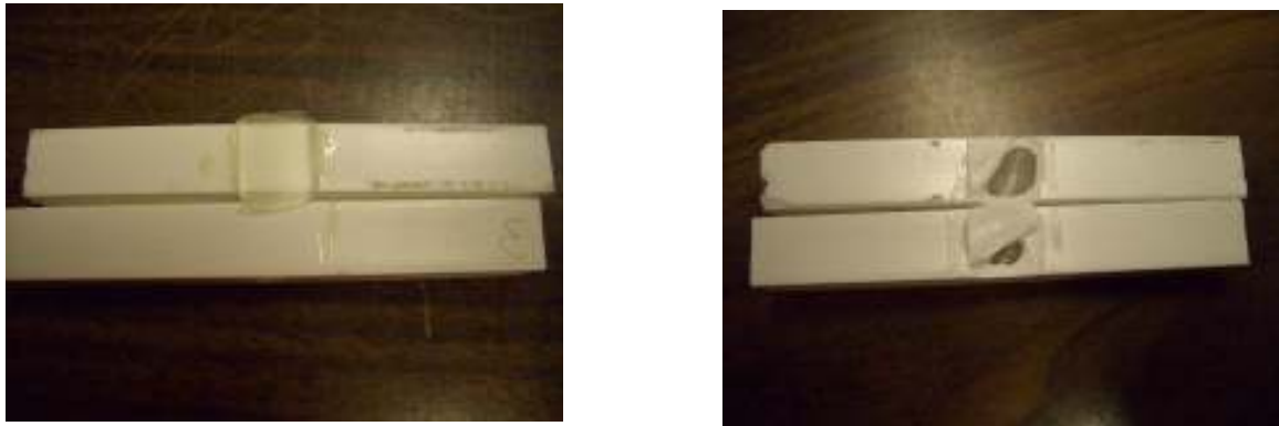
Figure 3: Epoxy and Cement Failure Modes (a) Epoxy Failure – adhesion failure (b) Polystyrene failure
